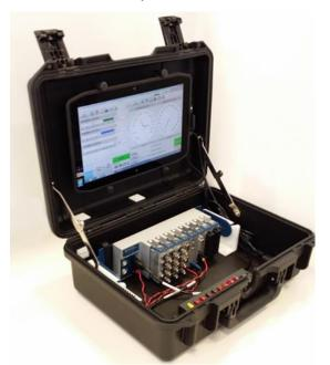
Complete in-vehicle DAQ system based on the National Instruments CompactDAQ platform.
