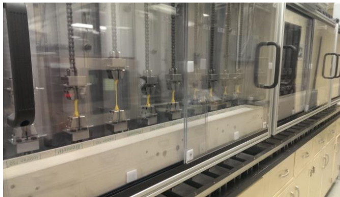
Figure 5: Creep tester samples on test
