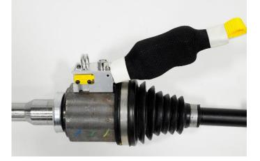
A hand-held sensor is attached magnetically to the half-shaft housing for quick and easy operator use.
