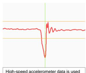
High-speed accelerometer data is used to verify half-shaft installation.
