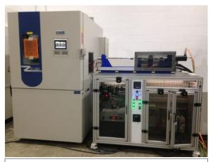
MDS developed this small motor test dynamometer including environmental simulation with support from Signal.X.
